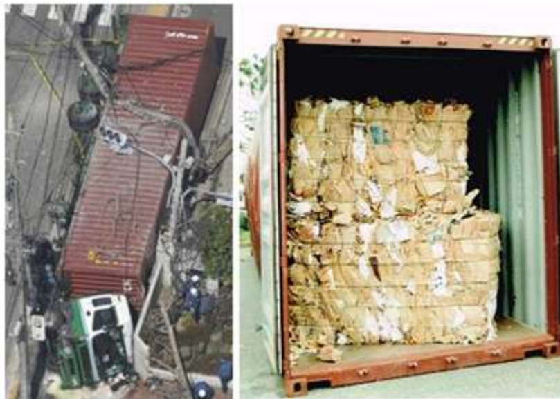
Figure 1: Trailer truck hauling a marine container in a typical rollover accident caused by a high center of gravity: March 25, 2014 at Tokyo Central.
