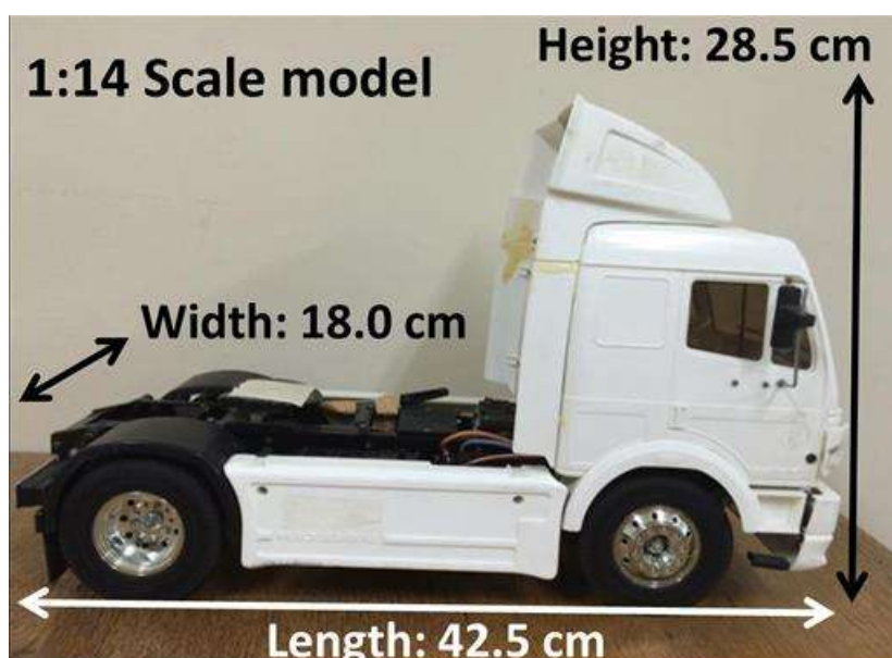
Figure 3: Model of truck to a scale of 1:14.
